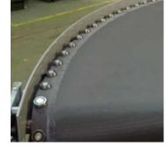
**Drive Position:** the preferred position for the drive unit is horizontally mounted on the outer radius at the discharge end of the belt bend. On some larger radius bends it is possible to vertically mount the geared motor on the inner radius.
