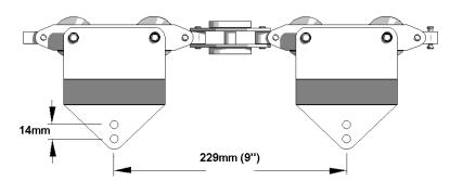
wheels are incorporated vertically and horizontally and are fitted with full compliment grade 100 steel ball bearings for optimum efficiency and trackability.
