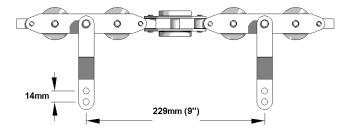
Incorporating medium duty pendants at 229mm pitch, the sturdy fully bi-planer chain includes articulating joints with cold rolled steel side plates. Double 41mm diameter wheels are incorporated vertically and horizontally and are fitted with full compliment grade 100 steel ball bearings for optimum efficiency and trackability.
