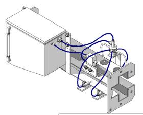
For long chain life, particularly when operating in high temperatures, lubrication is essential. The lubricator is a pneumatically powered unit which allows pulses of lubricant onto essential components. The unit includes a separate solenoid valve with silencer and regulator. Essential unit piping and connections would be preassembled and tested in our works.
