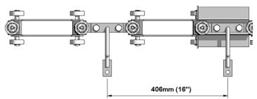
chain includes articulating joints with tensile steel side plates. Double 48mm diameter wheels are incorporated vertically and horizontally and are fitted with twin steel cage ball bearings for optimum efficiency and trackability.
