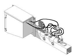
For long chain life, particularly when operating in high temperatures, lubrication is essential. The lubricator is a pneumatically powered unit which allows pulses of lubricant onto essential components. The unit includes a separate solenoid valve with silencer and regulator. Essential unit piping and connections would be pre-assembled and tested in our works.
