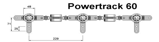
Incorporating medium duty pendants at 229 pitch, the sturdy fully bi-planer chain includes articulating joints with cold rolled steel side plates. Double 48mm diameter wheels are incorporated vertically and horizontally and are fitted with twin steel cage ball bearings for optimum efficiency and trackability.
