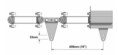
channels) and 5mm high tensile steel side plates. Double 48mm diameter wheels are incorporated vertically and horizontally and are fitted with steel cage ball bearings for optimum efficiency and trackability.
