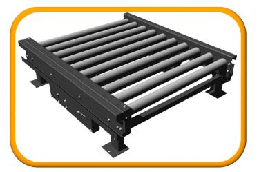
**Chain driven roller** modules with twin sprockets fully enclosed within the side channel. 76mm dia rollers at 155mm pitch providing a load capacity of 1500kg per pallet, the straight modules are able to handle upto 4500kg total conveyor load. Conveyor speeds of 12m/min or 18m/min. Support Stands available at a height to suit.
