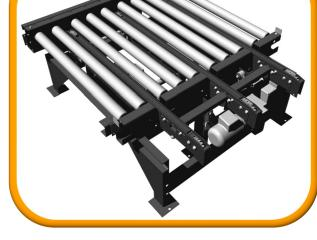
**Turntable module** is designed to change the direction of pallet travel by the rotation of the pallet through any angle from 90° to 180°, whilst keeping the relationship of the pallet runners to roller conveyor the same. 30 pallets per hour rotating 90 degrees.
