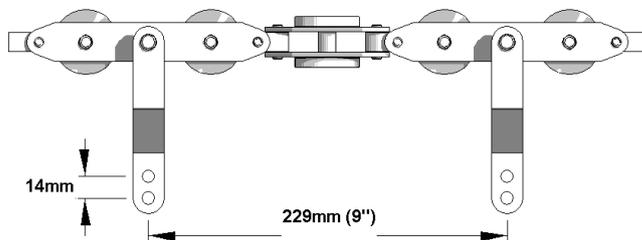
Incorporating medium duty pendants at 229mm pitch, the sturdy fully bi-planer chain includes articulating joints with cold rolled steel side plates. Double 41mm diameter wheels are incorporated vertically and horizontally and are fitted with full compliment grade 100 steel ball bearings for optimum efficiency and trackability.
