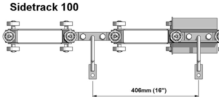
Double 48mm diameter wheels are incorporated vertically and horizontally and are fitted with twin steel cage ball bearings for optimum efficiency and trackability.
