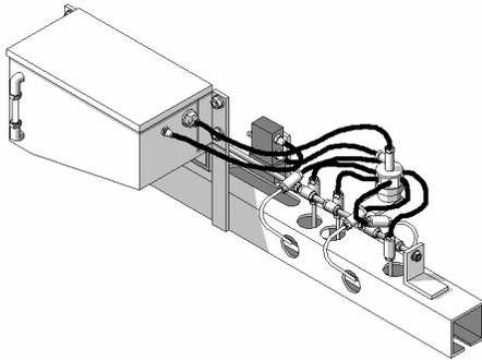
For long chain life, particularly when operating in high temperatures, lubrication is essential. The lubricator is a pneumatically powered unit which allows pulses of lubricant onto essential components. The unit includes a separate solenoid valve with silencer and regulator. Essential unit piping and connections would be pre-assembled and tested in our works.
