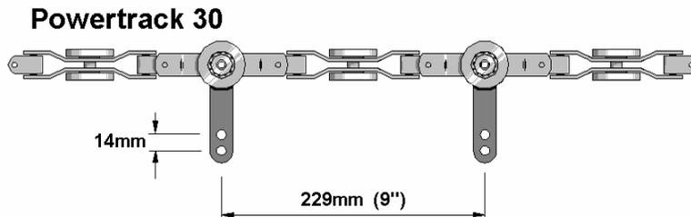
incorporated vertically and horizontally and are fitted with full compliment grade 100 steel ball bearings for optimum efficiency and trackability.
